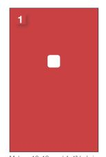
Make a 10x10 cm / 4x4" hole in the panel at the desired location for the center of your LCD.
